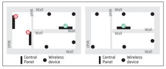
• The angle at which the transmitted signal hits the wall is very important. The effective wall thickness – and with it the signal attenuation – varies according to this angle. Signals should be transmitted as directly as possible through the wall.
