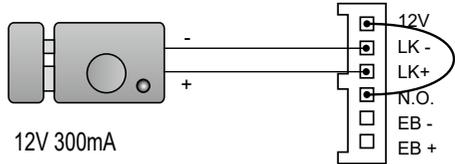
set to Normally open on the Unlock Relay mode
